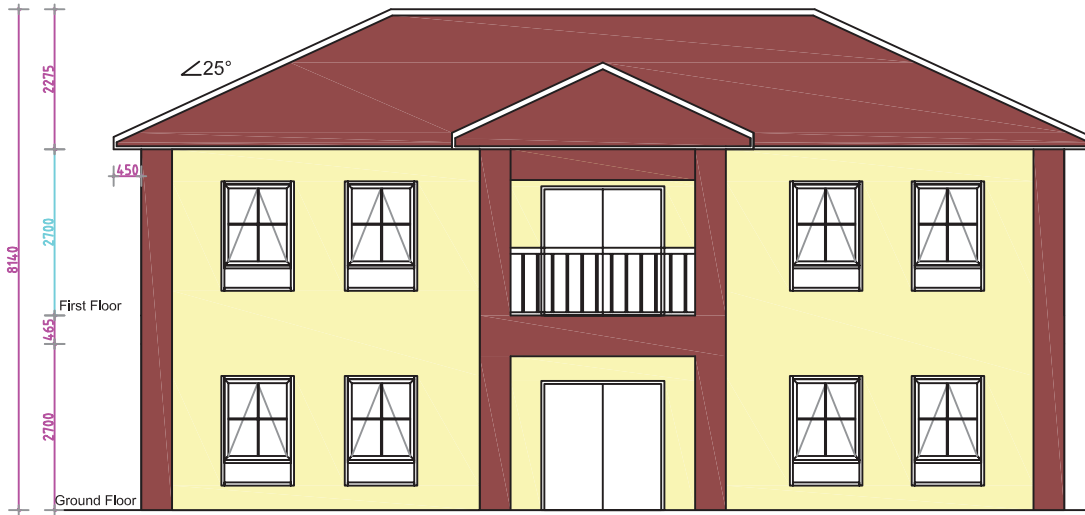
GABLE-FRONT ELEVATION SCALE 1:100
